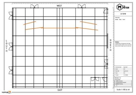
The lighting grid has fixed bars, and we can supplement this with extra scaff if needed.
